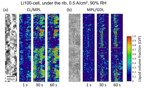
Fig. 8 Liquid water distribution under the rib: (a) at the CL/MPL interface and (b) at the MPL/GDL interface of the Li100-cell operated at 0.5 A cm<sup>-2</sup>, 90% RH; from left to right: dry state tomographic image, product water LVF distribution maps at 1, 30 and 60 s PEFC operation time. The Li-100 LVF distribution maps are more susceptible to artifacts (horizontal lines) than the VGCF ones, due to more difficult registration.
