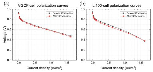
Fig. 2 Polarization curves of (a) VGCF-cell and (b) Li100-cell before X-ray exposure and after all nine tomographic scans; during polarization curve acquisition, cell temperature:  $45 \,^{\circ}$ C,  $H_2$ /air flow rate:  $200/200 \, \text{mL min}^{-1}$ , relative humidity (RH) of  $H_2$ /air: 100%/100%.
