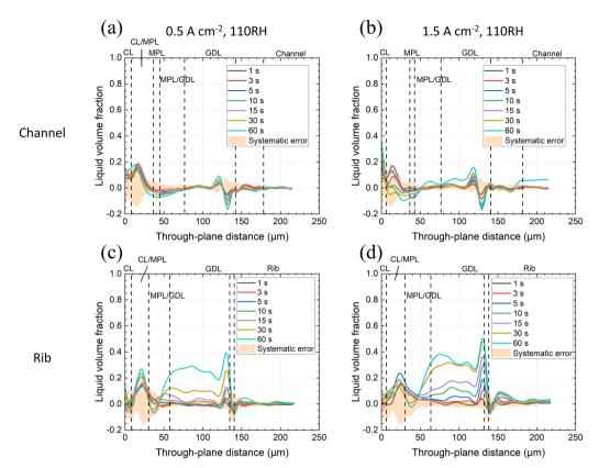
Different from the VGCF-cell, for the Li100-cell under the channel, the higher RH did not promote any water accumulation at the CL/MPL interface and in the MPL that was significant enough to be detected within the first minute of operation (Fig. 7a and b).
