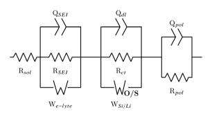
Fig. 3 ECs of symmetric and half-cells determined by fitting to EIS data
