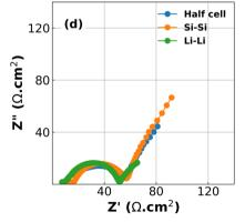
Fig. 1 EIS spectra collected for comparison between half cells and symmetric cells at (a) 0.2 V in the lithiation step; (b) 0.07 V in the lithiation step; (c) 0.3 V in the delithiation step; (d) 0.48 V in the delithiation step.
