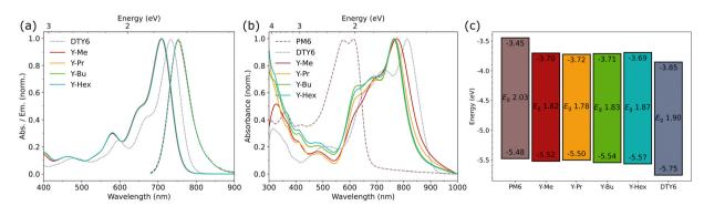
Fig. 1 (a) UV-Vis absorbance (solid lines) and emission (dashed lines) spectra in chloroform. (b) UV-Vis spectra of thin films. (c) Frontier molecular orbital energies and electrochemical bandgaps (Eq) determined from cyclic voltammetry measurements.
