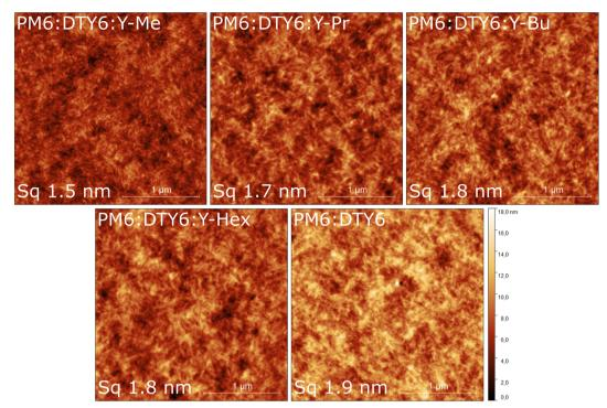
Fig. 4 AFM height images ( $2.5 \times 2.5 \, \mu m^2$ ) of the active layers of the ternary and binary blends prepared on glass/ITO/PEDOT:PSS substrates. The corresponding phase images are shown in Fig. S12 (ESI†).
