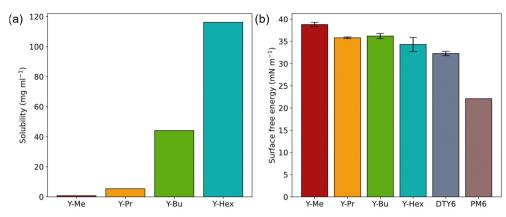
Fig. 2 (a) Solubilities of the acceptors in o-xylene at room temperature. (b) Surface free energy trends of the ternary setup components.
