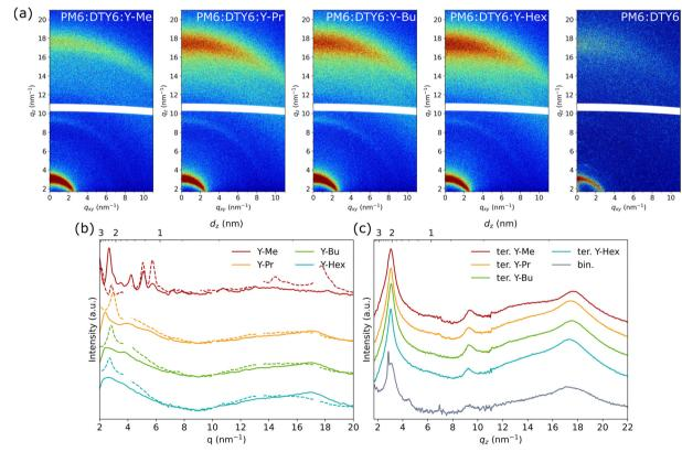
Fig. 5 GIWAXS characterization of drop cast films with thermal annealing treatment at 100 °C for 10 min. (a) 2D GIWAXS images of the ternary and binary donor:acceptor blends. 1D line cuts of (b) the neat acceptor films (in-plane  $(q_{xy})$  solid lines, out-of-plane  $(q_2)$  dashed lines), and (c) the ternary and binary donor:acceptor blends ( $q_z$  direction). The line cuts are shifted vertically for better visibility.
