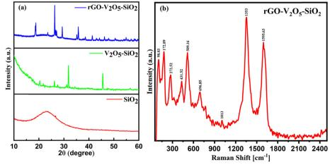
Fig. 3 (a) XRD spectra of rGO- $V_2O_5$ -SiO<sub>2</sub>,  $V_2O_5$ -SiO<sub>2</sub>, and only SiO<sub>2</sub> materials; (b) Raman spectra of the composite (rGO- $V_2O_5$ -SiO<sub>2</sub>) under the irradiation of a 532 nm laser
