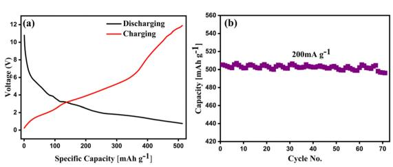
Fig. 6 (a) 12 V battery power supply at different specific capacities; (b) cycling performance of the 12 V battery at a constant current density of 200 mA g<sup>-1</sup>.
