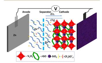
Fig. 1 Charge-discharge process with the structural alignment of the pouch cell describing the transportation of Zn<sup>2+</sup> ions in the presence of electrolyte with the cathode material.
