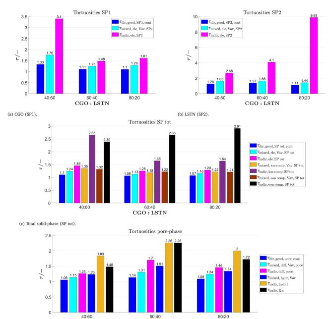
Fig. 14 Different tortuosities for (a) CGO (SP1), (b) LSTN (SP2), (c) total solid-phase (SP tot) and (d) the pore-phase for the LSTN-CGO dataset. The used variables are summarized in the Tables 6-8.
