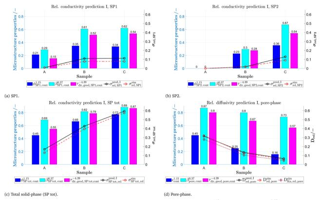
Fig. 24 M-factor prediction I (black lines) and its three components (volume fraction effect  $\phi^{1.15}$ , constrictivity effect  $\beta^{0.37}$  and tortuosity effect  $\tau_{\rm dir, qeod}^{-4.39}$ ) and simulated M-factors (red lines), for (a) SP1, (b) SP2, (c) total solid-phase (SP tot) and (d) the pore-phase of the sphere-packing structures. The used variables are summarized in the Tables 9 and 10.
