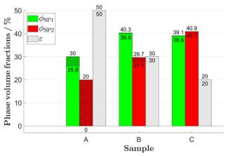
Fig. 20 Phase volume fractions SP1, SP2 and the pore-phase for the virtual sphere-packing structures. The discontiguous parts (islands/trapped pores) are hatched. The lower number corresponds to the contiguous phase and the upper number corresponds to the original phase volume fractions. Detailed definitions and description of the variables can be found in Table 1. Note that in Sample A, SP2 is fully discontiguous.
