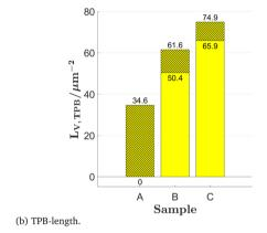
Fig. 21 (a) Volume specific interface areas and (b) TPB-length for the virtual sphere-packing structures. The disconnected parts (islands/trapped pores) are hatched. The lower number corresponds to the contiguous and the upper number corresponds to the original interface property. Detailed definitions and description of the variables can be found in Table 2.
