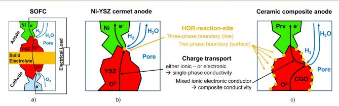
Fig. 1 Schematic visualization of SOFC electrodes: (a) working principle of a SOFC with a Ni-YSZ anode operated with hydrogen. Comparison of the conduction pathways and (simplified) reaction mechanisms of (b) a conventional Ni-YSZ anode and (c) an alternative perovskite (Prv)-CGO anode
