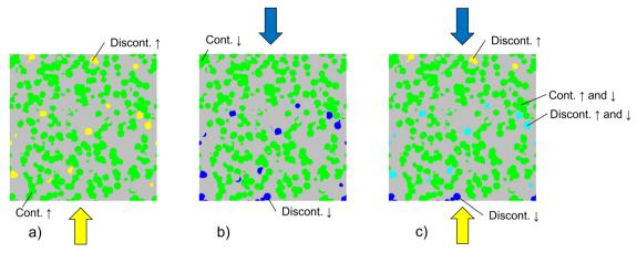
Fig. 4 Illustration of the contiguity analysis for the percolating SP1: (a) contiguity analysis from the bottom, (b) contiguity analysis from the top and (c) combined contiguous phase which is contiguous from the bottom and from the top.
