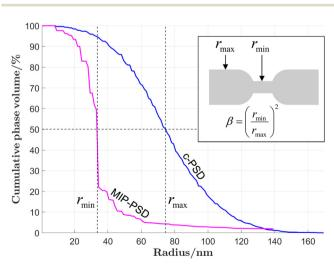
**Fig. 6** Illustration of the cumulative c-PSD and MIP-PSD curves for SP1 (CGO) of the CGO40–LSTN60 microstructure including the deduced properties  $r_{\text{max}}$  (mean radius of bulges),  $r_{\text{min}}$  (mean radius of bottlenecks) and  $\beta$  (constrictivity). Note: since MIP-PSD and c-PSD are determined by purely morphological analyses based on 3D images, they can be applied to any of the pore and solid phases.
