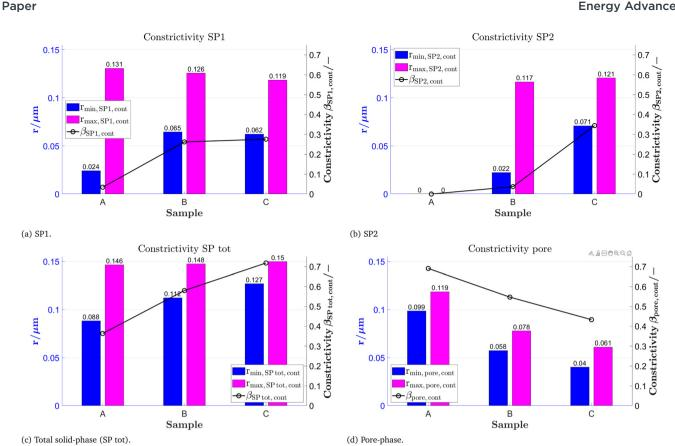
Fig. 22 Mean radius of bottlenecks  $r_{\text{min}}$ , mean radius of bulges  $r_{\text{max}}$  and corresponding constrictivity  $\beta$  for (a) SP1, (b) SP2, (c) total solid-phase (SP tot) and (d) the pore-phase for the sphere-packing structures. The used variables and their definitions are summarized in Table 5.
