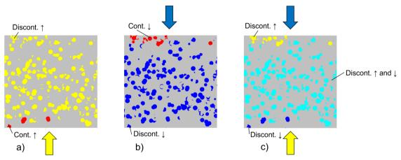
Fig. 5 Illustration of the contiguity analysis for the non-percolating SP2: (a) contiguity analysis from the bottom, (b) contiguity analysis from the top and (c) combination of the two analyses, which shows that there is no contiguous pathway in SP2 between top and bottom.
