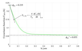
Fig. 7 Illustration of the characteristics of the covariance function for SP1 (CGO) of the CGO40–LSTN60 microstructure.  $\phi_{SP1}$  is the solid volume fraction of SP1 (CGO) and  $S_{V,SP1}$  is the total volume specific surface area of SP1, which is the sum of the two volume specific interface areas  $IA_{V,pore-SP1} + IA_{V,SP1-SP2}$ .
