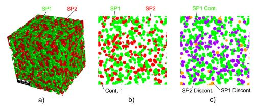
Fig. 3 Illustration of contiguity analysis for a monosized sphere structure that consists of two solid phases (SP1: green, SP2: red) and pores (white or transparent): (a) 3D-image, (b) 2D-orthoslice of the original microstructure and (c) contiguous (green) and discontiguous (orange) components of SP1 and discontiguous components (violet) of SP2 without any contiguous components.
