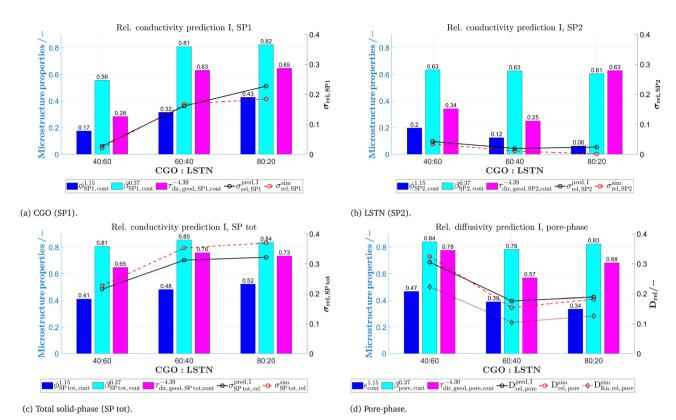
Fig. 15 M-factor prediction I (black lines) and its three components (volume fraction effect  $\phi^{1.15}$ , constrictivity effect  $\beta^{0.37}$  and tortuosity effect 439) and simulated M-factors (red lines), for (a) CGO (SP1), (b) LSTN (SP2), (c) total solid-phase (SP tot) and (d) the pore-phase. The used variables are summarized in the Tables 9 and 10
