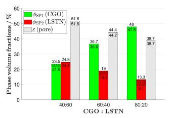
Fig. 10 Phase volume fractions of the CGO-phase (SP1), the LSTN-phase (SP2) and the pore-phase for the LSTN-CGO dataset. The discontiguous parts (islands/trapped pores) are hatched. The lower number corresponds to the contiguous phase and the upper number corresponds to the original phase volume fractions. Detailed definitions and description of the variables can be found in Table 1.
