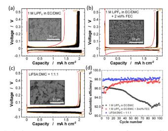
Fig. 3 Chronopotentiometric curves of Li deposition/stripping in Li/Cu cells with (a) 1 M LiPF<sub>6</sub> in EC/DMC, (b) 1 M LiPF<sub>6</sub> in EC/DMC + 2 vol% FEC and (c) LiFSA: DMC = 1:1.1 electrolyte solutions at a current density of  $0.35~\mathrm{mA~cm^{-2}}$ . SEM images of Li metal deposited on the Cu electrode at a current density of 0.35 mA cm<sup>-2</sup> for 6 h are also shown in the inset of (a-c). (d) Coulombic efficiency of Li deposition/stripping in each cell.
