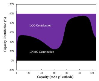
Fig. 6 Simulated capacity contribution from LCO (purple) and LNMO (black) at C/20 discharge (1.13 mA cm<sup>-2</sup>) for the 45%LCO cathode AAM electrode cell
