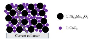
Fig. 1 Cartoon illustrating the LiCoO<sub>2</sub> (LCO) network in a multicomponent AAM electrode facilitating electronic conductivity through the electrode matrix. Larger black dots and smaller purple dots represent the LiNi<sub>0.5</sub>Mn<sub>0.5</sub>O2 (LNMO) and LCO particles, respectively. The green line depicts a relatively low resistance electronic conduction path from the current collector to a LNMO particle far from the current collector via the LCO network in the AAM electrode.
