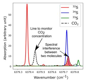
Fig. 5 Simulated spectra showing the S-isotopologue lines of H<sub>2</sub>S and interfering CO2 lines in the spectral region covered by the VCOF-CRDS setup
