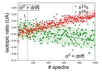
Fig. 4 Time series of isotopic ratio measurements (3 s per spectra) reveal a spectral interference between H<sub>2</sub>S and other outgassed molecules [CO<sub>2</sub> lines are observed in 'old' gas (Fig. 5)]. This sets a limit to the experimental repeatability
