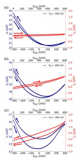
Fig. 2 I-V transfer characteristics of the rGO device featuring the (a) pristine Au, (b) cCu-modified Au gate, (c) pCu-modified Au gate recorded in Milli-Q water. The red curve stands for the leakage current (I<sub>G</sub>) and the blue one stands for the current recorded at the P terminal  $(I_P)$ .  $V_P = 0 \text{ V}$  and  $V_{\rm N}$  = -300 mV.  $V_{\rm GP}$  and  $V_{\rm GN}$  = ( $V_{\rm G}$  -  $V_{\rm N}$ ) ranges are presented as the bottom and top x-axis, respectively.
