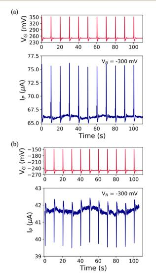
Fig. 4 Emulated AP iterative series (red lines) and its recorded AP iterative series (blue lines) featuring (a) +250 mV set point potential and (b) -250 mV set point potential in NaCl 0.1 M
