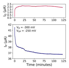
Fig. 5 (a)  $I_{\rm G}$  and (b)  $I_{\rm P}$  vs. time plots for the prolonged electrical stress investigation, in which  $V_{\rm N}$  = -300 mV and  $V_{\rm GP}$  = -250 mV were fixed in 0.1 M NaCl.
