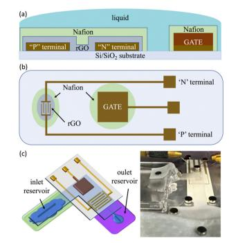
Fig. 1 (a) Vertical cross-section and (b) top view sketches of the EGT. (c) Sketch and photograph of the paper fluidic setup applied on the Cu-gated devices for long measurements by fluxing 0.1 M NaCl.
