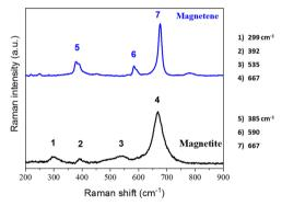
Fig. 9 Representative Raman spectra of magnetite and Magnetene nanoplatelet samples.
