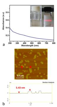
Fig. 8 (a) UV-Vis spectrum of magnetene in water. The inset photo shows magnetene dispersion in water (Tyndall effect). (b) AFM image and the height profile of magnetene nanoplatelets.
