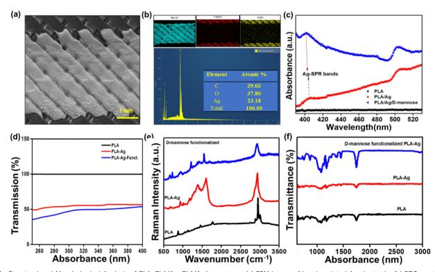
Fig. 2 Structural and Morphological Analysis of PLA, PLA/Ag, PLA/Ag/D-mannose (a) SEM image of brush-painted Ag electrode. (b) EDS spectra and elemental color mapping of PLA-Ag electrode. (c) Absorbance spectra, (d) transmission %, (e) Raman spectra, and (f) FTIR spectra of neat PLA, PLA/Ag, PLA/Ag/p-mannose
