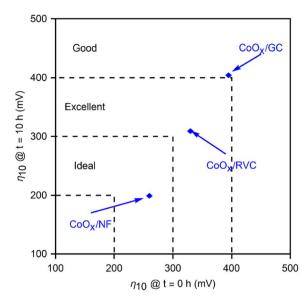
Fig. 10 Parametric plot of the overpotentials at a current density of 10 mA cm $^{-2}$  at the start of polarization (x-axis) and at t=10 h (y-axis) for three  $CoO_x$  films deposited on the three substrates: GC, RVC and NF, as well as the shaded regions representing where the  $(Ni/Co/FeO_x)$  films deposited on different substrates fall. The dashed lines catalogue different activity regions into qualitative terms. All reported values are for the OER performed in 1.0 M KOH.
