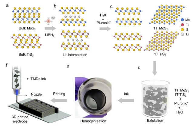
Scheme 1 Schematic representation of the synthesis process, exfoliation mechanism and 3D printing of 1T'/1T MoS<sub>2</sub>/TiS<sub>2</sub> inks. (a) Atomic structures of bulk MoS<sub>2</sub> and TiS<sub>2</sub> and (b) atomic lattices of lithiated MoS<sub>2</sub> and TiS<sub>2</sub>. (c) and (d) Pluronic-water exfoliation process of MoS<sub>2</sub> and TiS<sub>2</sub>. (e) Homogenization of 1T'/1T MoS<sub>2</sub>/TiS<sub>2</sub> inks and (f) extrusion of the corresponding inks through a nozzle.
