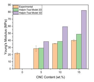
Fig. 7 The comparison of the experimental Young's modulus data of PA36,9/CNC nanocomposites with the theoretical values from the Halpin-Tsai models with 2D and 3D randomly dispersed fillers
