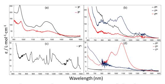
Fig. 5 (a): NIR spectra for  $2^U$  (4.6 mM in Tol) and  $3^U$  (3.0 mM in THF). (b): vis-NIR spectra for the  $1^{Np}$ ,  $2^{Np}$  and  $3^{Np}$  series. (0.69 mM in Tol, 0.50 mM in Tol and 2.1 mM in THF respectively). (c): vis-NIR spectra for  $3^{Pu}$  (1.0 mM in THF). (d): vis-NIR spectra of  $3^{Ce}$ ,  $2^{Ce}$  and  $1^{Ce}$  (9.51 mM, 5.86 mM and 2.32 mM respectively) in toluene.
