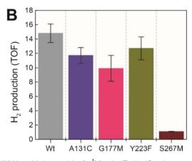
Fig. 4 (A)  $H_2$  oxidation activity (s $^{-1}$ ) for the TmHydS variants measured at 70 °C in 200 mM phosphate buffer pH 8 under a 100%  $H_2$  atmosphere following 1 mM benzyl viologen reduction using UV-vis absorbance at 600 nm. (B)  $H_2$  production activity (s $^{-1}$ ) measured at 70 °C with gas chromatography after 10 min of incubation with 100 mM sodium dithionite and 10 mM methyl viologen.
