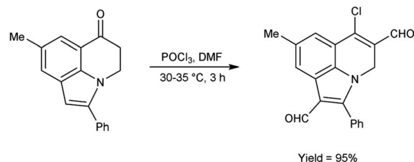
Scheme 47 Synthesis of 6-oxo-6H-pyrrolo[3,2,1- ij ]quinoline-1,5-dicarbaldehyde.
