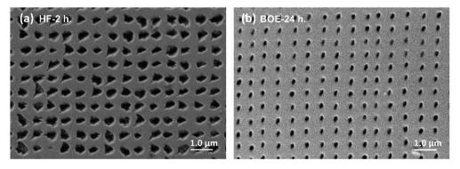
Fig. 2 Comparison of the sample surface by using 40% HF (a) and BOE (b) in chemical etching. The pulse energy in prior laser writing is 11 nJ. The etching time is 2 hours and 24 hours for 40% HF and BOE, respectively.
