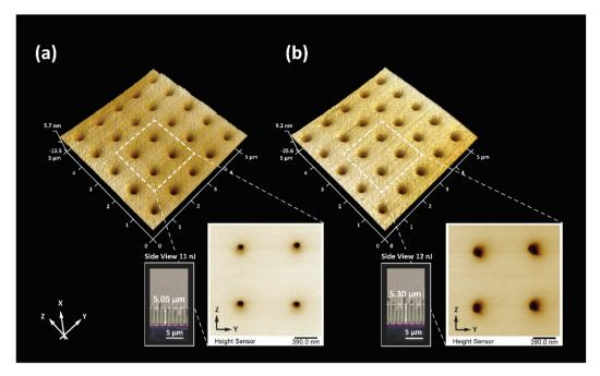
Fig. 4 The AFM images of the sample surfaces by using pulse energies of 11 nJ (a) and 12 nJ (b). The etching time is 2 hours. The insets are the optical images of the side view of the structure. The average etching depths are  $5.05 \mu m$  and  $5.30 \mu m$ , respectively.
