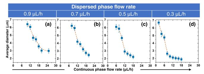
Fig. 4 Relationship between QD-MB diameter and continuous flow rates. The dispersed flow rate was set at 0.9 μL h<sup>-1</sup> (a), 0.7 μL h<sup>-1</sup> (b), 0.5 μL h<sup>-1</sup> (c), and 0.3 µL h<sup>-1</sup> (d). Increasing the continuous flow rate led to a decrease in the average diameter of QD-MBs. The coefficient of variance for the size distribution was less than 10%.
