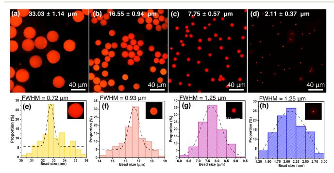
Fig. 2 Fluorescence micrographs and size distribution of QD-MBs of different sizes, depending on the flow rate. (a-d) Micrographs of QD-MBs with average diameters of 33.03 μm, 16.55 μm, 7.75 μm, and 2.11 μm, respectively. (e-h) Corresponding size distribution histograms of the QD-MBs.
