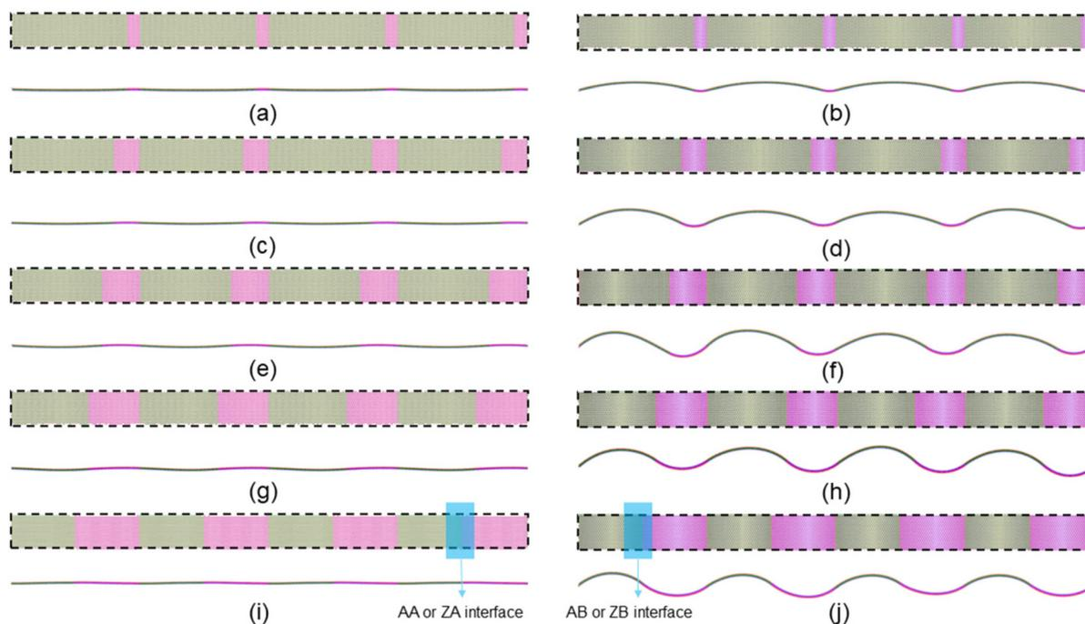
**Fig. 2** The top and side views of optimized (a, c, e, g, and i) AA and (b, d, f, h, and j) AB Janus MoSSe/WSSe heterostructures with  $L_m/L_n$  as (a and b) 1/9, (c and d) 2/8, (e and f) 3/7, (g and h) 4/6, (i and j) 5/5, respectively.
