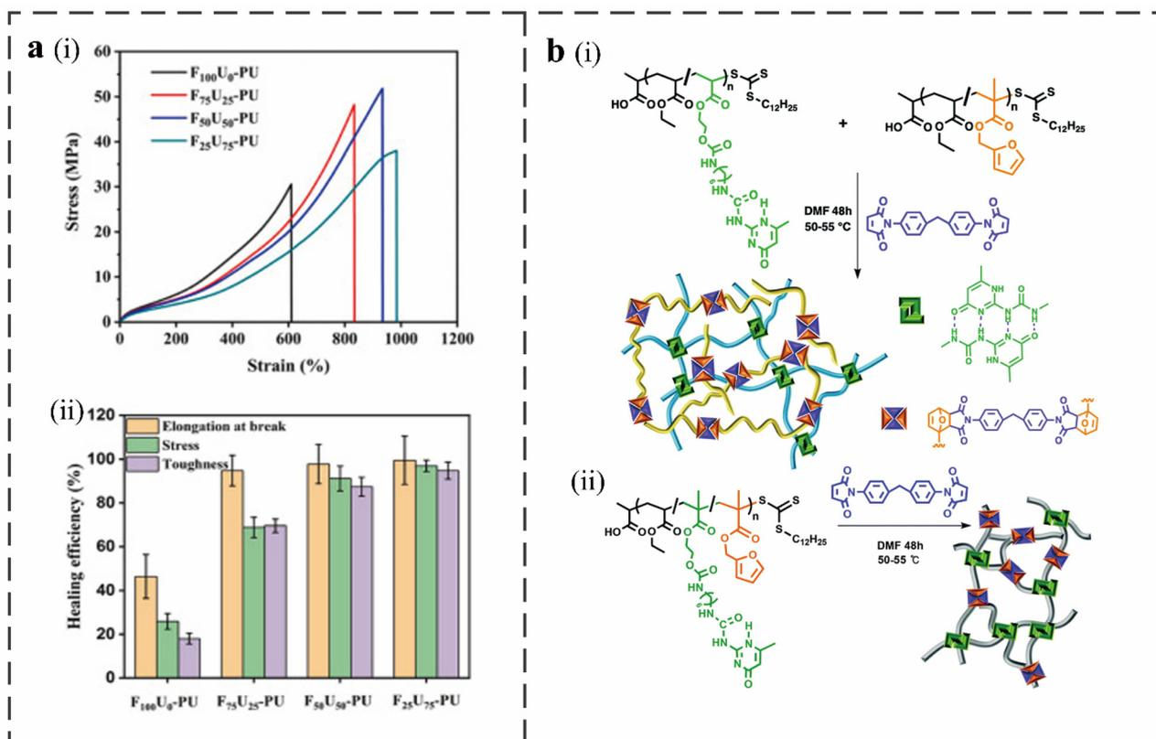
Fig. 4 (a), (i) Typical stress–strain curves of FaUb-PU. (ii) Healing efficiency of breaking strain, stress, and toughness of FaUb-PU.<sup>3</sup> (b) Crosslinkers and polymers used in the preparation of RAFT based IPN (i) and SN (ii) materials. Slashes indicate random incorporation of monomers.<sup>9</sup>
