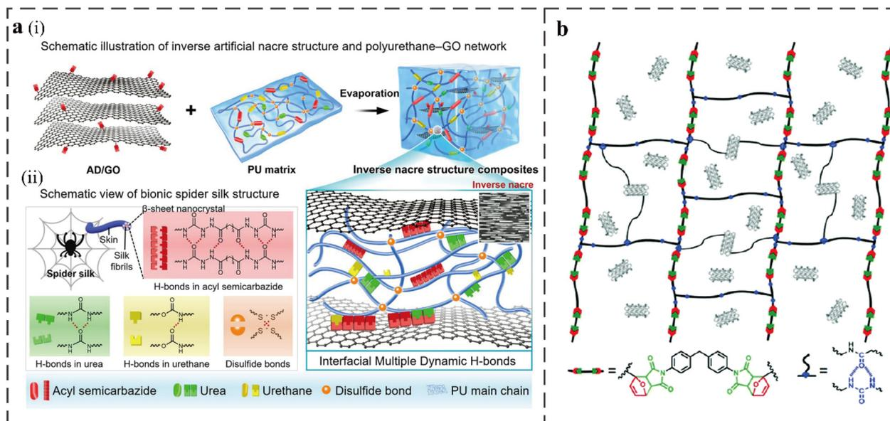
**Fig. 7** (a) (i) Schematic of the PU–graphene oxide network with an inverse artificial nacre structure. (ii) Dynamic bond interaction in the biomimetic composite.<sup>2</sup> (b) The structure of cross-linked networks of RCFA.<sup>6</sup>
