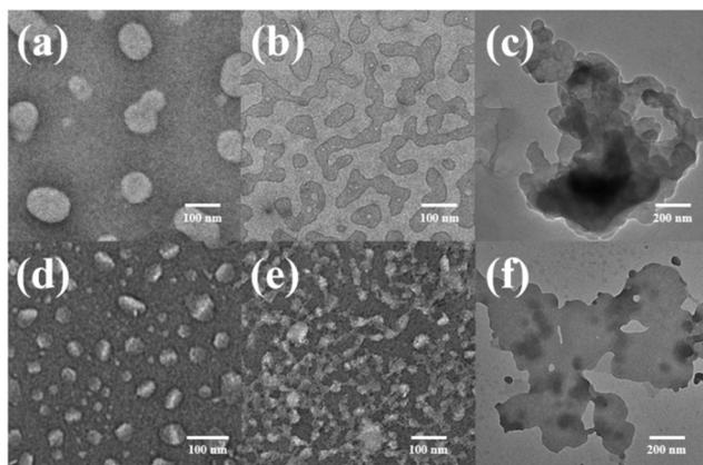
**Fig. 9** TEM images of molecule **H**<sub>1</sub>**C****G** (c/c = 4 : 1) obtained from CHCl<sub>3</sub>/DMSO (v/v = 19 : 1) solutions after (a) 1 h, (b) 4 h and (c) 24 h. TEM images of molecule **H**<sub>2</sub>**C****G** (c/c = 4 : 1) obtained from CHCl<sub>3</sub>/DMSO (v/v = 19 : 1) solution after (d) 1 h, (e) 4 h and (f) 24 h.
