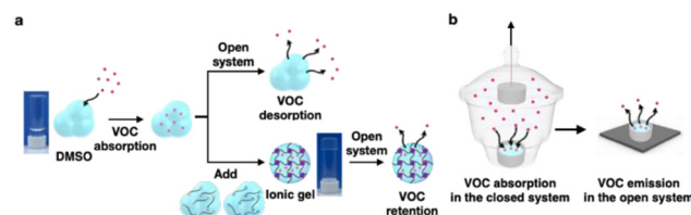
Fig. 5 (a) Mechanism of the absorption and desorption of VOCs from the DMSO and mechanism of the retention of the VOCs through forming an ionic gel. (b) Schematic of experimental conditions in the open system.
