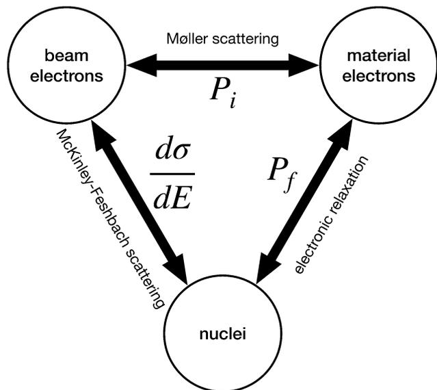
**Fig. 1** Three interactions between three pairs of particles involved in electron beam-induced sputtering. In insulators, the probability of material electronic excitation ( $P_i$ ) and the probability that those excitations are substantially long-lived ( $P_f$ ) can be large. Therefore, the effect of exciting the material electrons on the sputtering rate should not be ignored in these materials.
