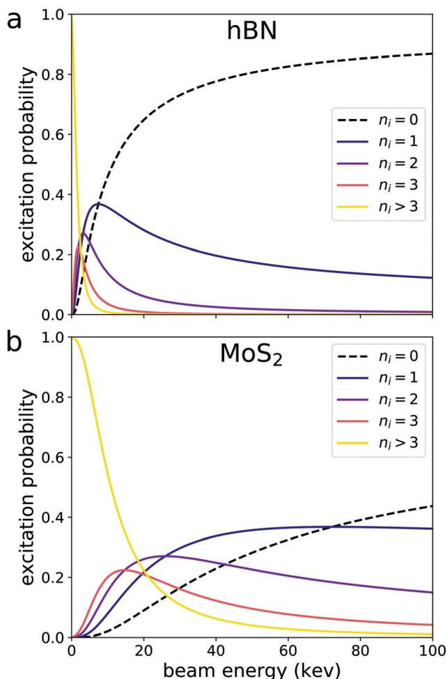
**Fig. 3** Probabilities of initially exciting a certain number of electrons  $n_i$  in (a) hBN and (b) MoS<sub>2</sub> with a beam electron. The excitation probabilities tend to decrease with increasing beam energy. The excitation probabilities in MoS<sub>2</sub> are larger than those in hBN because MoS<sub>2</sub> has a significantly smaller band gap.
