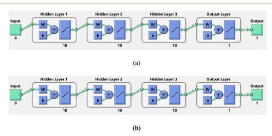
Fig. 13 Neural network for (a) heat transfer and (b) mass transfer.
