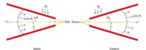
Fig. 1 Geometrical configuration.
