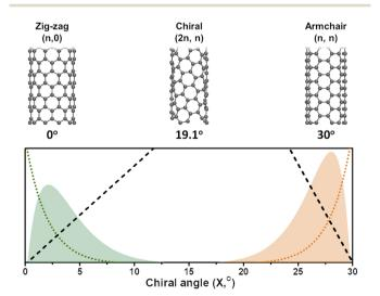
Fig. 1 (Bottom panel) The SWCNT population distributions (y-axis) calculated as a product of nucleation probability (dotted) and the growth rate (dashed) shown for near ZZ (green) and near-AC (orange) chiralities (similar to ref. 22), and (top panel) the schematic of the SWCNTs corresponding to the chiral angles shown below.
