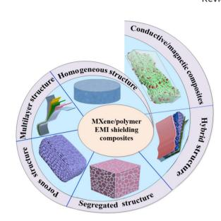
Fig. 1 Structural design of MXene/polymer EMI-shielding composites.
