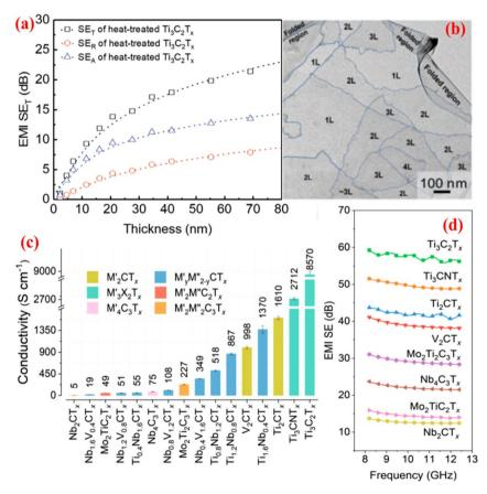
Fig. 2 (a) EMI SE values of  $Ti_3C_2T_x$  film after annealing at 400 °C and (b) transmission electron microscopy image of few-layer thick MXene film. Reproduced with permission from ref. 62 with permission from Wiley-VCH Verlag GmbH & Co. KGaA, Weinheim, © 2020. (c) Conductivity and (d) EMI SE of 5  $\mu$ m-thick MXene films with different compositions. Reproduced from ref. 63 with permission from the American Chemical Society, © 2020.
