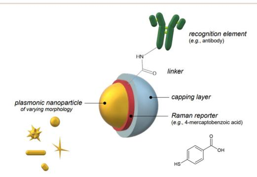
Fig. 12 Schematic representation of the components of a SERS nanotag: a plasmonic nanoparticle of varying morphology (yellow), an embedded or chemisorbed Raman reporter (red), a biocompatible capping layer (e.g., silica, a polymer such as polyethylene glycol or bovine serum albumin, etc.; pale blue), and a recognition element such as an antibody (green), covalently conjugated to the Raman reporter via the use of a linker molecule. The SERS nanotag components are not in scale.
