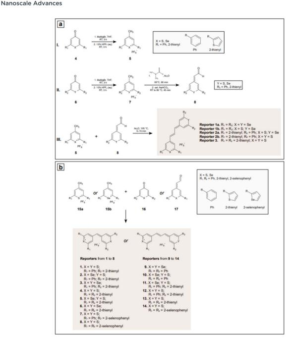
Scheme 2 (a) Reaction scheme for the synthesis of 785 nm-resonant chalcogenpyrylium reporters as prepared by Harmsen et al.<sup>231</sup> Abbreviations: THF, tetrahydrofuran; RT, room temperature; Ph, phenyl; Ac<sub>2</sub>O, acetic anhydride; sat., saturated. (b) Precursors and final chalcogenpyrylium reporters active under 1280 nm excitation, as prepared by Bedics et al.<sup>233</sup>
