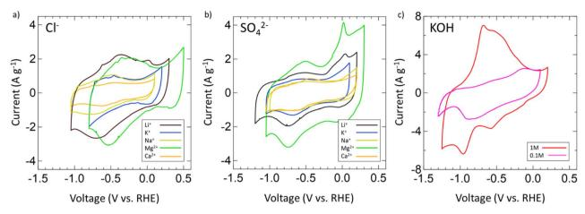
Fig. 3 CVs of operating voltage windows for (a) chlorides, (b) sulfates of  $Mg^{2+}$  (green), Li<sup>+</sup> (black), K<sup>+</sup> (blue), Na<sup>+</sup> (yellow), and Ca<sup>2+</sup> (orange) at 50 mV s<sup>-1</sup>. (c) CVs for 1 M (red) and 0.1 M (pink) KOH. All chlorides and sulfates are 1 M concentration except for K<sub>2</sub>SO<sub>4</sub> (0.5 M), CaSO<sub>4</sub> (0.06 M), and CaCl<sub>2</sub> (0.02 M) due to low solubility at room temperature.
