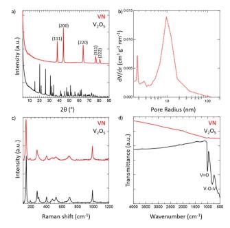
Fig. 1 Physical characterization of high surface area passivated VN powder using (a) XRD for bulk characterization, (b)  $N_2$ -physisorption for pore size distribution, and (c) Raman and (d) FTIR spectroscopies for surface characterization.
