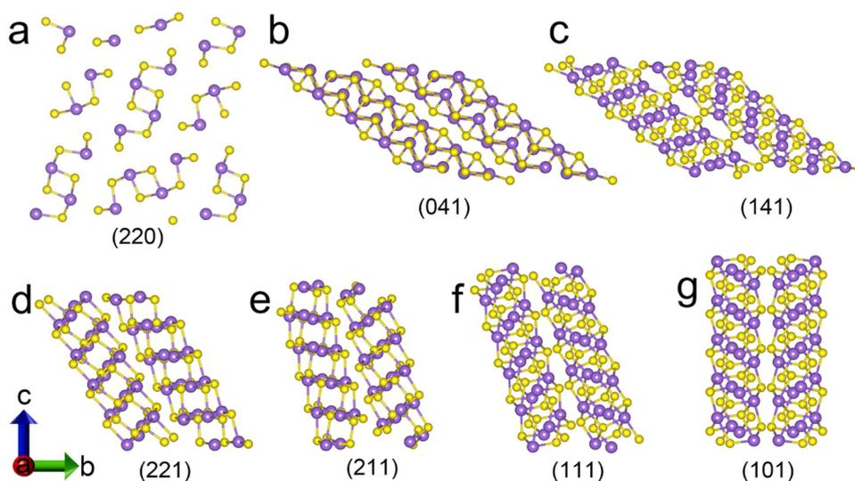
Fig. 16 Schematic of the  $(\text{Sb}_4\text{Se}_6)_n$  ribbons with different crystal planes ( $\text{Sb}^{3+}$  = purple dots and  $\text{Se}^{2+}$  = yellow dots). Adapted with permission from ref. 1 Copyright 2022, Elsevier Ltd.
