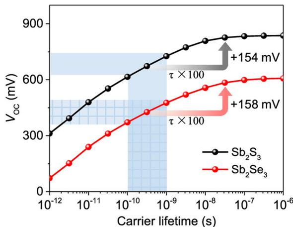
Fig. 14 Simulated  $V_{OC}$  of  $Sb_2S_3$  and  $Sb_2Se_3$  solar cells as a function of carrier lifetime by SCAPS. The shadow area exhibits the generally accepted lifetimes and  $V_{OC}$  of the  $Sb_2S_3$  and  $Sb_2Se_3$  solar cells. Adapted with permission from ref. 29 Copyright 2020, the American Chemical Society.
