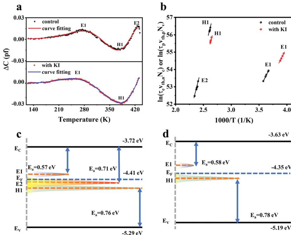
Fig. 8 (a) DLTS signals for the device without and with KI post-treatment. (b) Corresponding Arrhenius plots obtained from the DLTS signals. Position distribution of CBM ( $E_C$ ), VBM ( $E_V$ ), Fermi level ( $E_F$ ) and defect energy level for  $Sb_2(S,Se)_3$  films (c) without and (d) with KI post-treatment. Adapted with permission from ref. 85 Copyright 2022, Wiley-VCH.
