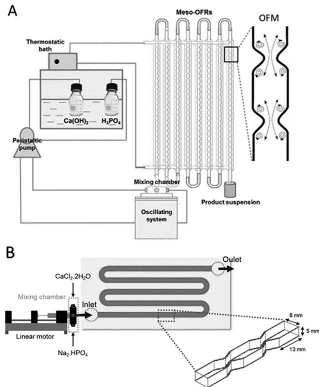
Fig. 2 (A) Scaled-up meso-OFRs and oscillatory flow mixing inside a reactor and (B) MOFPR used for continuous manufacturing of HAP particles.<sup>14,17</sup>
