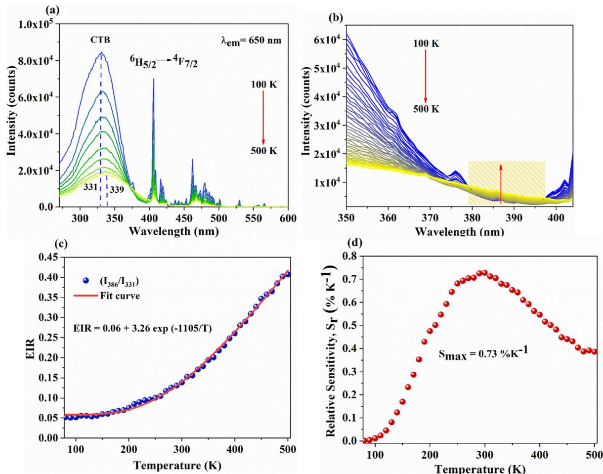
Fig. 8 (a) The TDPLE spectra monitored under emission at 560 nm, (b) the zoomed view of the CTB edge of the TDPLE spectra, and (c) and (d) the variation of EIR and relative temperature sensitivity,  $S_r$ , with temperature.
