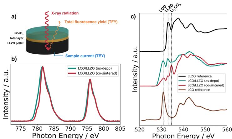
Fig. 3 (a) Schematic of the XAS measurement geometry, (b) Co  $L_{2,3}$ -edge, and (c) O K-edge in fluorescence mode (TFY) for LLZO, LCO, and 50 nm LCO|LLZO as-deposited and annealed at 500 °C in oxygen.
