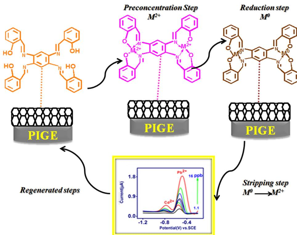
Scheme 1 Mechanism of  $[\text{Pb}^{2+}$  and  $\text{Cd}^{2+}\text{-TSAB}]/\text{MWCNT}$  electrode.
