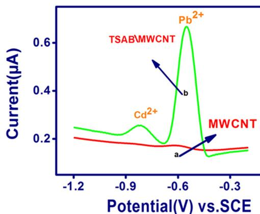
**Fig. 3** SWASV performed on MWCNT (A) and TSAB/MWCNT (B) with Pb<sup>2+</sup> and Cd<sup>2+</sup> (8 ppb) accumulated on electrode surface in 0.1 M acetate buffer solution (pH 5.5).
