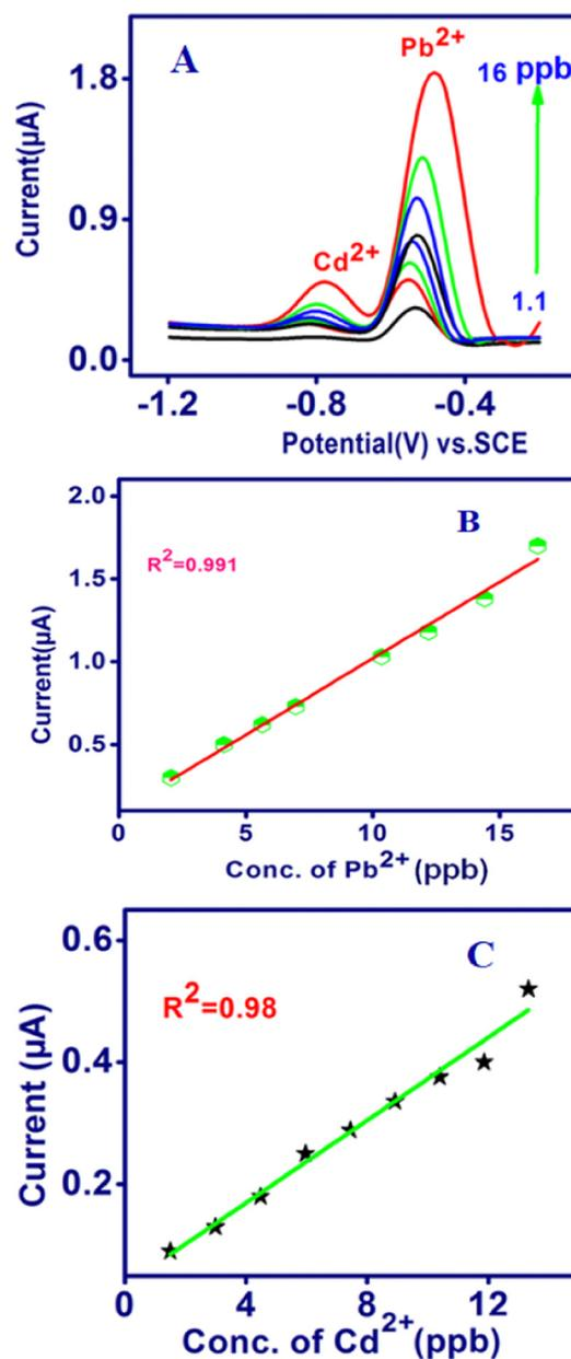
Fig. 5 Simultaneous determination of  $\text{Pb}^{2+}$  and  $\text{Cd}^{2+}$  by TSAB/MWCNT using (A) SWASV. Corresponding calibration plots for  $\text{Pb}^{2+}$  (B) and  $\text{Cd}^{2+}$  (C) calculated using SWASV.
