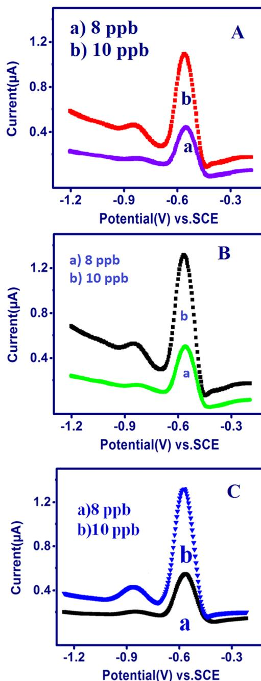
Fig. 8 SWASV of the TSAB/MWCNT in pH 5.5 ABS containing a 10 ppb mixture of  $\text{Pb}^{2+}$  and  $\text{Cd}^{2+}$  at an  $E_{\text{acc}}$  of  $-1.2$  V and  $T_{\text{acc}}$  of 240 s in a few environmental samples: honey (A), raw milk (B) and groundnut shell (C).
