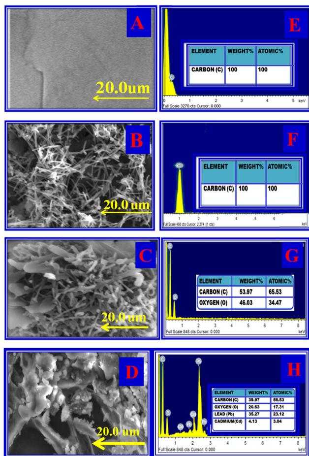
Fig. 1 Surface morphology. SEM image of PIGE (A), MWCNT (B), TSAB/MWCNT (C), and  $[\text{Pb}^{2+}$  and  $\text{Cd}^{2+}\text{-TSAB}]/\text{MWCNT}$  (D). EDAX image of PIGE (E), MWCNT (F), TSAB/MWCNT (G) and  $[\text{Pb}^{2+}$  and  $\text{Cd}^{2+}\text{-TSAB}]/\text{MWCNT}$  (H).
