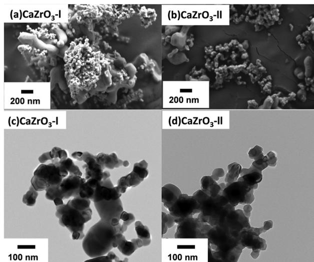
Fig. 4 SEM (a), (b) and TEM (c), (d) images of CaZrO<sub>3</sub>-I and CaZrO<sub>3</sub>-II.
