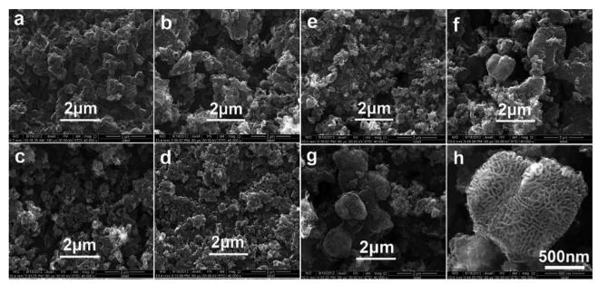
Fig. 14 SEM images of carbon powders obtained under cell voltages of 3.0 V (a), 3.5 V (b), 4.0 V (c), 4.5 V (d), 5.0 V (e), 5.5 V (f), (h) and 6.0 V (g) at 450 ° C in Li<sub>2</sub>CO<sub>3</sub>-Na<sub>2</sub>CO<sub>3</sub>-K<sub>2</sub>CO<sub>3</sub> mixture.<sup>71</sup>
