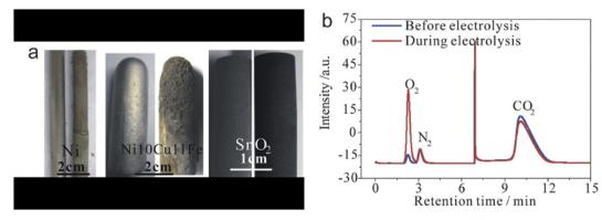
Fig. 10 (a) Digital photos of Ni,  $Ni_{10}Cu_{11}Fe$  and  $SnO_2$  electrodes before and after serving as the anode; (b) gas chromatograms of the outlet gas before and during electrolysis using the  $SnO_2$  anode.<sup>35</sup>
