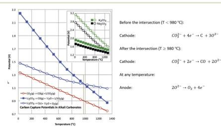
Fig. 5 Electrochemical conversion potential for carbon capture and conversion centra Li<sub>2</sub>CO<sub>3</sub> (main figure), or Na<sub>2</sub>CO<sub>3</sub> or K<sub>2</sub>CO<sub>3</sub> (figure inset); in the inset, squares refer to  $M_2CO_3 \rightarrow C + M_2O + O_2$  and circles to  $M_2CO_3 \rightarrow CO + M_2O + \frac{1}{2}O_2$ . To the right of the brown vertical line, CO is preferred. And C is preferred to the left of the line.<sup>74</sup>
