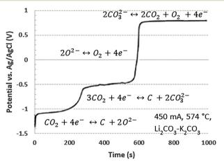
Fig. 13 Chrono-potentiometric plots for anodic oxidation of the electro-deposited carbon in Li<sub>2</sub>CO<sub>3</sub>-K<sub>2</sub>CO<sub>3</sub> at 574 °C, reproduced from ref. 41 with open-access permission from the Royal Society of Chemistry, copyright 2014.
