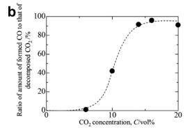
Fig. 16 (a) Amounts of decomposed CO<sub>2</sub> gas and produced CO gas as a function of inlet gas flow rate; (b) ratio of the amount of formed CO gas to that of decomposed CO<sub>2</sub> gas as a function of the initial gas concentration of CO<sub>2</sub>. 42
