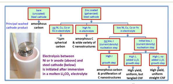
Fig. 8 Molten carbonate electrolysis pathways converting CO<sub>2</sub> leading to high yield, uniform CNF product. 92
