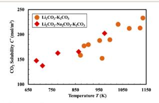
Fig. 7  $\,^{\circ}$  CO $_2$  solubility in molten carbonates at different temperatures at 1.01  $\times$  10<sup>5</sup> Pa. $^{87}$
