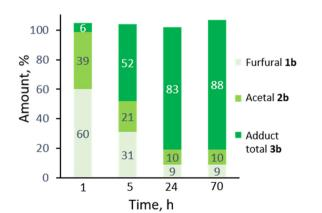
Fig. 2 Profile of the one-pot acetalization/DA in time (20 equiv. allyl alcohol, TFA 10 mol%, 3 Å MS, 100 °C).
