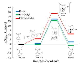
Fig. 3 DFT mechanism (calculated with B3LYP at 6-311+g(d) and GD3BJ dispersion, in methanol (SMD)); only the paths leading to the *anti*-3 adducts were calculated; blue = furfuryl allyl ether 2a; green: furfural diallyl acetal 2b; red: intermolecular reaction between furfural and allyl alcohol; GS = ground state, RC = reactive conformation.
