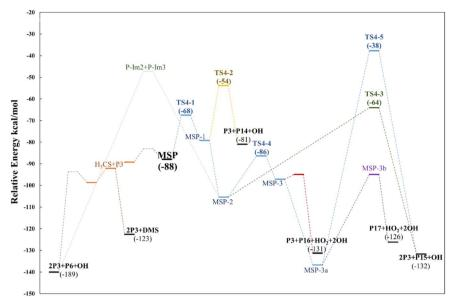
Fig. 14 Relative energy diagram for decomposition of the MSP intermediate formed in the AMS oxidation initiated by OH radicals in the absence of  $NO_x$  at the M06-2X/GD3/auq-cc-pVTZ level.
