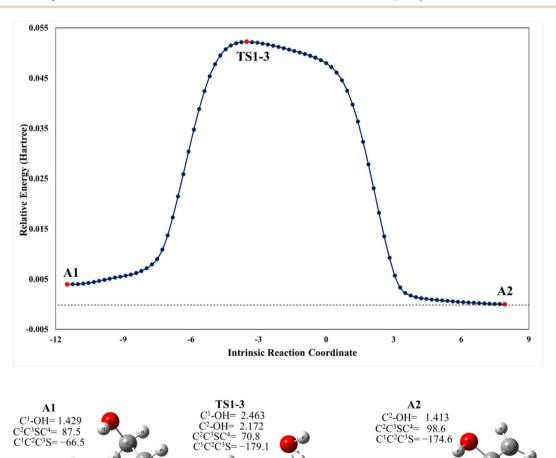
Fig. 4 Upper panel: a plot of intrinsic reaction coordinates for the transition state between the A1 and A2 intermediaries, TS1-3. Lower panel: optimized structures at the M06-2X/GD3/aug-cc-pVTZ level (XYZ coordinates of these species are collected in the ESI†).
