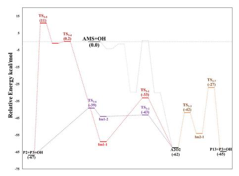
Fig. 12 Relative energy diagram for decomposition of the A2O2 intermediate (addition to C2) formed in the AMS oxidation initiated by OH radicals in the absence of  $NO_x$  at the M06-2X/GD3/aug-cc-pVTZ level.
