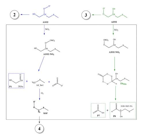
Fig. 7 General mechanism for decomposition of  $RO_2$  radicals formed in the AMS oxidation initiated by OH radicals in the presence of  $NO_x$ . Proposed products are shown enclosed in dashed line boxes.
