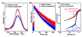
Fig. 2 (a) PL spectra, (b) TRPL and (c) trap density of perovskite without (control) and with (target) APDI.
