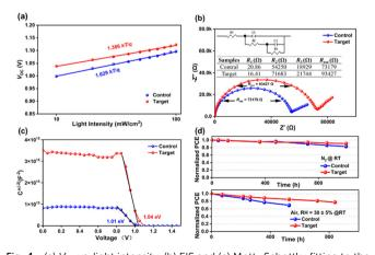
Fig. 4 (a)  $V_{\rm oc}$  vs. light intensity, (b) EIS and (c) Mott-Schottky fitting to the capacitance-voltage plots for the control and target devices. (d) Stability of unencapsulated devices under N2 and air conditions.
