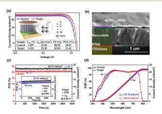
Fig. 3 (a) J-V curve of PSCs and the illustration of device structure based on ADPI modification, (b) cross-sectional SEM image of PSC, (c) stabilized power output at the maximum power point under AM 1.5G and (d) EQE for the control and target devices.
