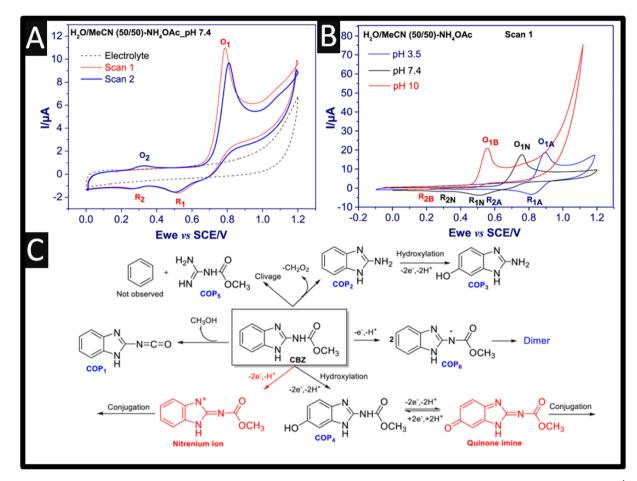
Fig. 1 (A) Cyclic voltammograms of 1 mM carbendazim in  $H_2O/MeCN$  50 : 50 with 0.1 M ammonium acetate pH 7.4, scan rate 50 mV s<sup>-1</sup>, and (B) cyclic voltammograms of 1 mM carbendazim at three different pH (Basic, B; Neutral, N and Acidic, A). (C) the main chemical species observed after the electrochemical oxidation of carbendazim. Figures reproducible from ref. 9. Copyright 2021 Elsevier.
