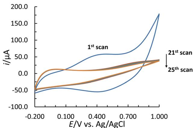
**Fig. 4** Measured CV voltammograms during the removal of insulin (electrocleaning approach) from the formed Ppy matrix in  $0.01$  M PBS ( $\text{pH } 7.2$ ) with a  $\nu$  of  $50$   $\text{mV s}^{-1}$ .
