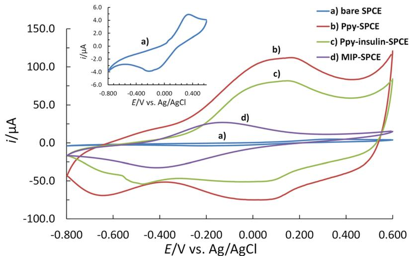
**Fig. 5** The electrochemical behaviour of the step-by-step imprinting process in 0.01 M PBS (pH 7.2) containing the 5 mM  $[\text{Fe}(\text{CN})_6]^{3-/4-}$  redox probe using the CV: (a) the bare SPCE (blue solid line), (b) the Ppy-SPCE (red solid line), (c) the Ppy-insulin-SPCE (green solid line), and (d) the MIP-SPCE (purple solid line). The measurements were performed at a  $\nu$  of  $50 \text{ mV s}^{-1}$ . The insert shows the CV voltammogram of a bare SPCE at a lower  $i$  scale.
