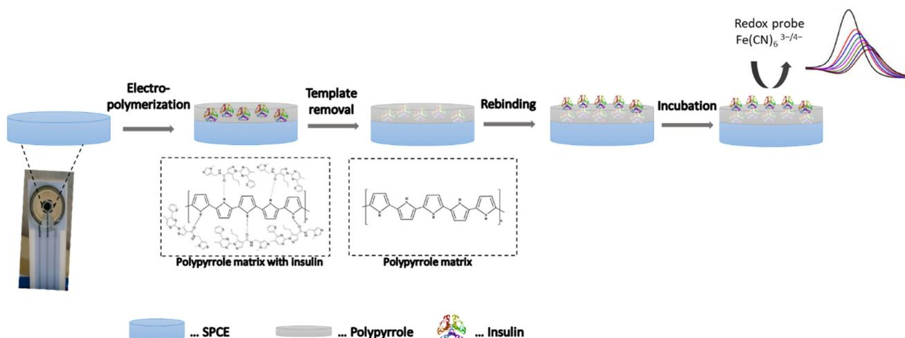
**Fig. 1** A schematic depiction of insulin imprinting on the surface of the SPCE. The overall process involved (1) the electrosynthesis of Ppy in the presence of the template molecule (insulin), (2) the removal of the target protein by electrocleaning, and (3) the determination of the rebinding ability of the formed molecular imprinted polymer film (MIP-SPCE) by using a standard redox probe and SWV.
