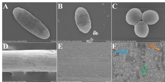
**Fig. 2** SEM of (A to C) single bacteria (from left to right: V.P, S.T, S.A), (D) single gold stirring rod and (E) its surface, (F) gold stirring rod simultaneously enriched three target pathogenic bacteria.
