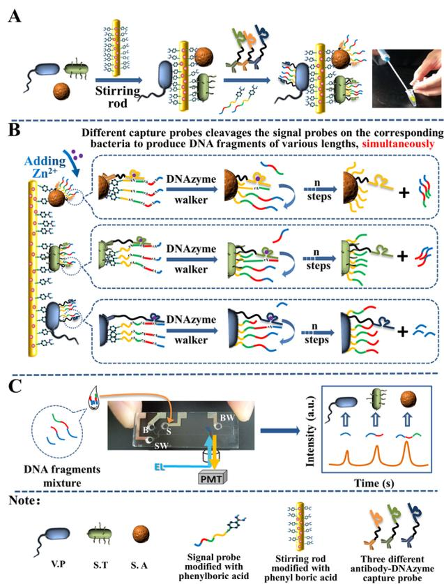
**Scheme 1** The principle of the multivalent DNA walker sensor Au-Rods @ PBA @ Bacteria @ DNA-Walker to simultaneously detect three pathogenic bacteria.
