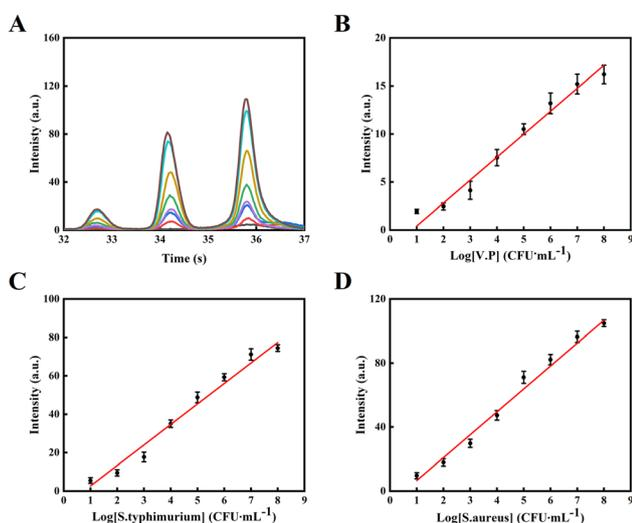
**Fig. 6** (A) Microfluidic chip technology determination of V.P, S.T, and S.A in the concentration range from  $10$  CFU mL<sup>-1</sup> to  $1 \times 10^8$  CFU mL<sup>-1</sup>. (B), (C), and (D) Correspond to the calibration plots for V.P, S.T, and S.A, respectively. (The signal probe was  $0.2 \mu\text{M}$  and the capture probes were  $0.02 \mu\text{M}$ , pH was 8.0, the reaction buffer was PBS buffer, and time was 0.5 h).
