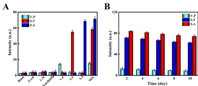
**Fig. 5** (A) The selectivity performance of the sensor with the interference of different bacteria. (B) Stability of the biosensor. (The concentration of bacteria was  $1 \times 10^6$  CFU mL<sup>-1</sup>, pH was 8.0, the reaction buffer was PBS buffer and time was 0.5 h).
