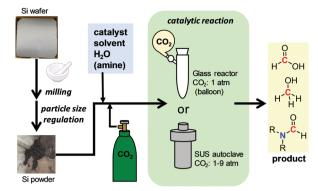
Fig. 2 Method for catalytic CO<sub>2</sub> reduction with powdered Si wafer.
