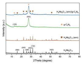
Fig. 2 XRD patterns of the as-prepared  $H_4Nb_6O_{17}$  before and after annealing at 300  $^{\circ}\text{C}$  and g-C<sub>3</sub>N<sub>4</sub> and their composites samples
