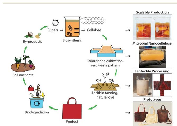
**Fig. 1** Microbial biofabrication and green processing of minimal waste products with a closed-loop life cycle (left). Right: scalable MC production from different carbon sources, including fructose (beaker A) and sucrose (beaker B); lecithin tanning and biocoloration of textiles biosynthesized to the geometry of a design pattern, to create products, such as our bioleather bag prototypes, that meet performance and biodegradability criteria for a circular economy.
