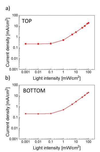
Fig. 4 Linearity (current density vs. light power) of the semitransparent (ITO top contact) MA<sub>0.3</sub>FA<sub>0.7</sub>Pb<sub>0.5</sub>Sn<sub>0.5</sub>I<sub>3</sub> perovskite photodetector illuminated from the (a) top and (b) bottom.
