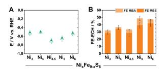
Fig. 2 Half-cell potentials of the herein investigated Ni<sub>x</sub> pellet electrodes after 2 h of electrolysis at 100 mA cm<sup>-2</sup> (A). The respective faradaic efficiency values via GC-MS quantification (B).
