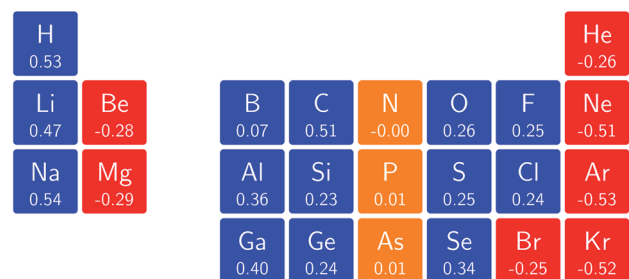
Fig. 10 Initial responses of the hardness in a magnetic field as a periodic table representation showing both the numerical values and categorising them with a color code in which blue indicates a positive derivative, red a negative derivative and yellow a derivative that is zero or close to zero.
