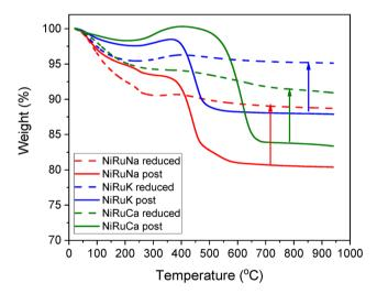
$\label{eq:Fig. 16} \textbf{TGA} \ \ \text{for reduced and post reaction NiRuNa}, \ \ \text{NiRuK} \ \ \text{and NiRuCa} \ \ \text{samples}.$
