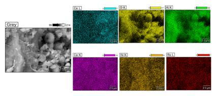
Fig. 13 SEM and EDX mapping of NiRuCa.
