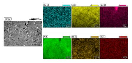
Fig. 11 SEM and EDX mapping of NiRuNa.
