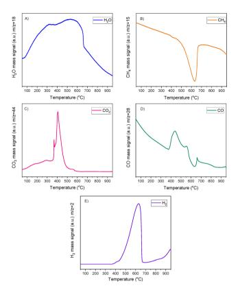
Fig. 7 CH<sub>4</sub>-TPSR profile of NiRuCa: (A) H<sub>2</sub>O, (B) CH<sub>4</sub>, (C) CO<sub>2</sub>, (D) CO and (E) H<sub>2</sub> signals.
