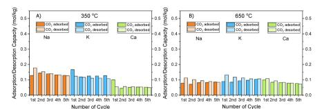
Fig. 3 CO<sub>2</sub> Adsorption/desorption cycles of Na, K and Ca at (A) 350 °C and (B) 650 °C.
