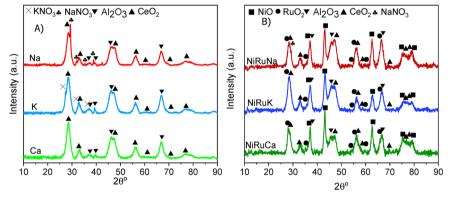
Fig. 9 XRD patterns of the fresh (A) supported adsorbents and (B) DFMs.
