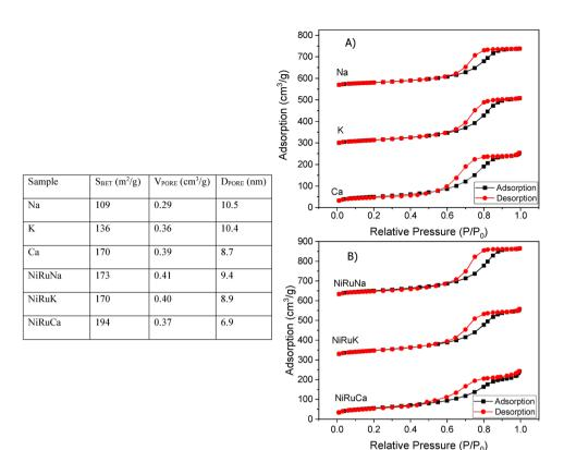
Fig. 8 Textural properties of the materials on the left-hand side and nitrogen adsorption—desorption isotherms of the (A) supported adsorbents and (B) DFMs on the right-had side.
