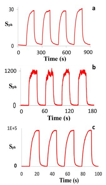
**Fig. 4** The photo-response characteristics of the (a) ZNWA-based, (b) single ZNW-based, and (c) ZNL-based PDs.
